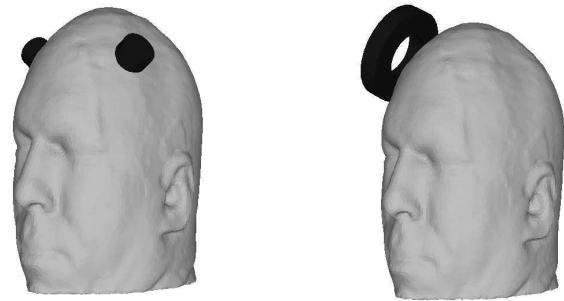
Fig. 1. The ideas of ECT (left) versus TMS (right): in ECT two metallic electrodes are placed on the skin and head is subjected to voltage pulses up to several hundreds volts; in TMS a coil operating in pulse mode is placed close to the head.
